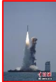
Fig.4: This is the first time that China has succeeded in the "one-stop" marine launch of a carrier rocket. The assembly, various checks, port hauling, and launch processes have been integrated, reducing mission completion times by a third.
