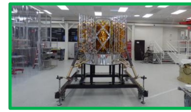
図-7：AstroboticsのPeregrine着陸機(アセンブリの後半フェーズ)写真(Credit: SpaceNews/Jeff Foust) [NO.083]
