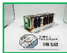
Fig.14: The IHI-SAT, a 3U-sized microsatellite equipped with the AIS reception system; main mission is to demonstrate AIS functions
