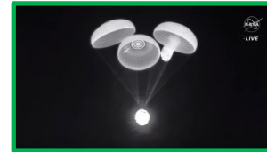
Fig.9: Infrared image of the Crew Dragon's descent for the Crew-2 mission. One of four parachutes is not fully deployed. (Credit: NASA TV)
