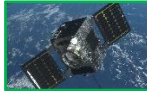
Fig.5: The HawkEye 360 satellite launched in December 2020 is significantly larger than the older model and includes processor updates and a larger solar array for increased onboard power for multiple simultaneous signal acquisition. (Photo credit: HawkEye 360)
