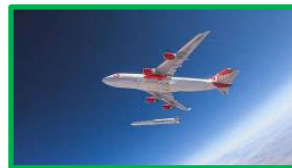
Fig.16: Rocket launched separately in-sky from an aircraft (Credit: Provided by ANA Holdings) (Copyright Jiji Press)
