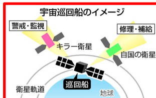
Fig.16: Conceptual overview of the "space patrol vessel" planned by Japan's Ministry of Defense, featuring alerts/surveillance and satellite repair functions
