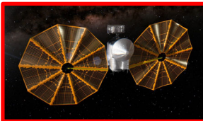
Fig.4: "Lucy" conceptual image; one solar array might not be able to be fully deployed. (Credit: NASA's Goddard Space Flight Center)
