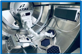
Fig.19: Robot for assembling solar panels developed by GITAI Japan (no.105)
