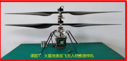
Fig.3: Prototype for a Mars surface cruise drone developed by NSSC in China (credit: NSSC/CAS) (no.007)
