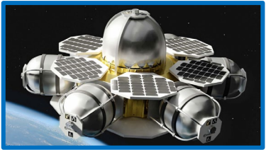
Fig.12: Design concept of Orbit Fab's Tanker-002 (credit: Orbit Fab) (no.108)
